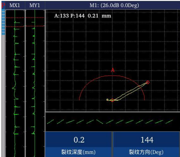
Figure 2 Defect at 144 degree
